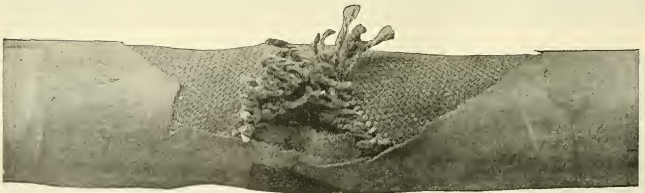
Showing cheap grade of Air-Brake Hose made by competitor, where it burst at the end of the shank of the coupling.
